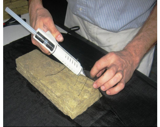
3. Center the QuietFiber material over fabric* and apply the hot glue as desired.
