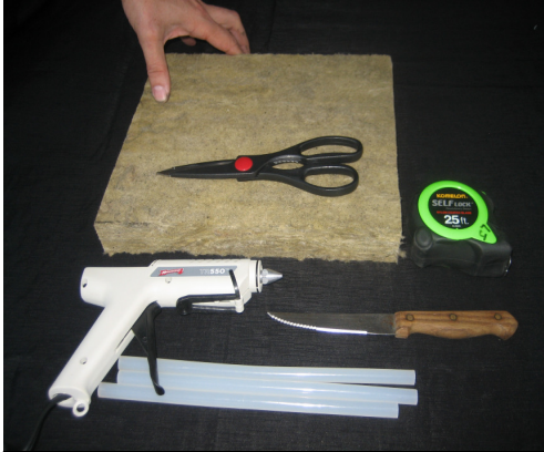
1. Materials needed for QuietFiber install. Hot glue gun, scissors, fabric*, serrated knife, measure
