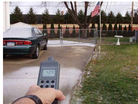
After installation of Acoustifence, decibel readings at the Coca Cola plant dropped from 89 decibels to 68 decibels ( left ) and at a neighboring residence ( right ).
