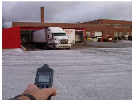
After installation of Acoustifence, decibel readings at the Coca Cola plant dropped from 89 decibels to 68 decibels ( left ) and at a neighboring residence ( right ).
